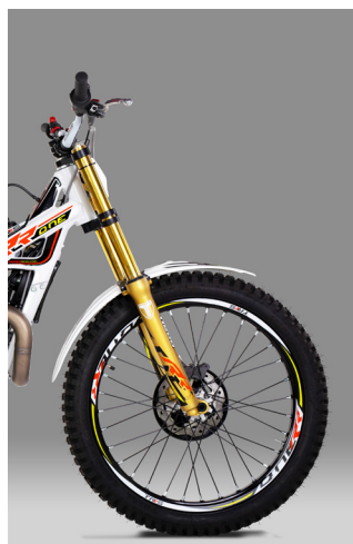
a) On the right-hand side of the suspension you can set the preload.
