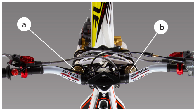
a) Spring preload; b) Adjusting the length
